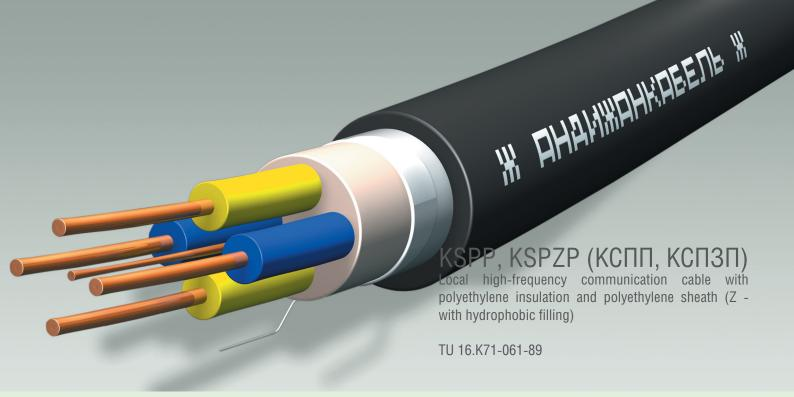
The cable is designed for inter-station and subscribers communication with transmission systems with time division of channels and pulse-code modulation of up to 2048 Kbit/sec speed with DC voltage of remote power of up to 500 V.
