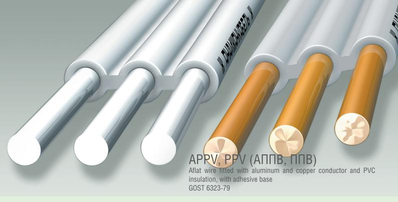
The wire is designed for electric plants and fixed installation in power lighting systems, as well as for fixed installation of electrical equipment of apparatuses, mechanisms and machines at rated voltage of up to 450 V (for 450/750 V networks) and frequency of up to 400 Hz or DC voltage of up to 1000 V. The wire is not intended for flexible installation.
