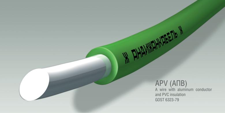
The wire is designed for electric plants and fixed installation in power lighting systems, as well as for fixed installation of electrical equipment of apparatuses, mechanisms and machines at rated voltage of up to 450 V (for 450/750 V networks) and frequency of up to 400 Hz or DC voltage of up to 1000 V.
