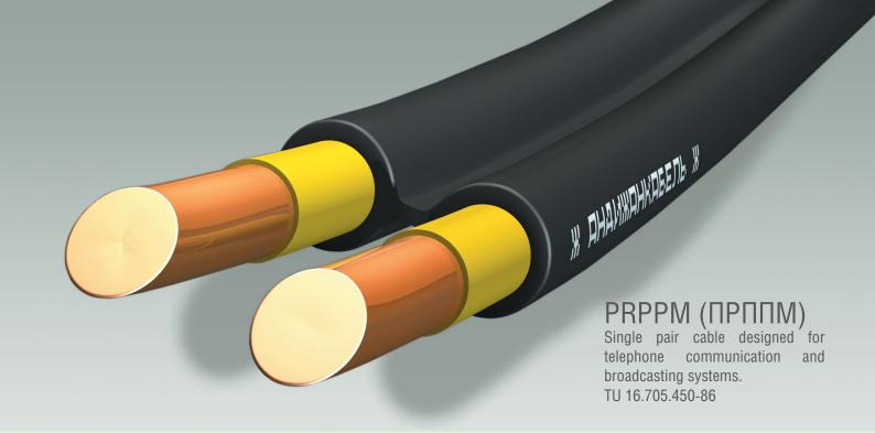
Single pair cable for telephone communication and broadcasting systems is designed for operation at voltage of up to 380 V and frequency of up to 10 kHz at subscriber lines of telephone communication systems and wire broadcasting distribution networks.
