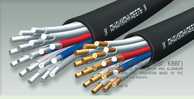
The cable is designed for fixed connection to electrical devices and equipment, as well as for installation of terminals of switch stations with rated AC voltage of up to 660 V, up to 100 Hz frequency and DC voltage of up to 1000 V.
