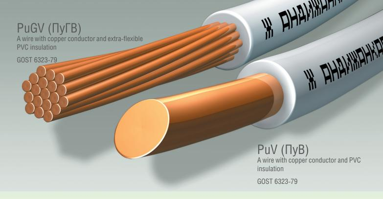
The wire is designed for electric plants at fixed installation in lighting and power systems, as well as for fixed installation of electrical equipment, apparatuses, mechanisms and machines at rated voltage of up to 450 V (for 450/750 V networks) and frequency of up to 400 Hz or DC voltage of up to 1000 V.
