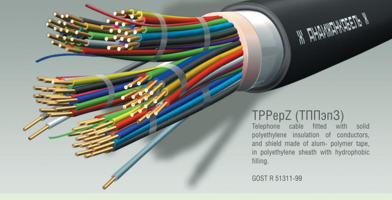
Installation in telephone ducts, conduits and wells; installation along building walls; hanging on overhead communication lines in high humidity conditions.
