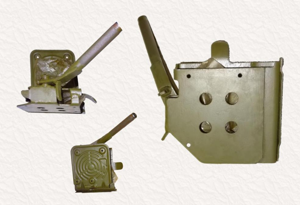
The device allows you to simplify and speed up the process of preparing a machine gun ammunition belt for use. Consists of flat base, case of complex configuration with two clamp brackets, sleekers, along which the machine-gun ammunition belt passes, lever handle, pushing mechanism and pawl.
