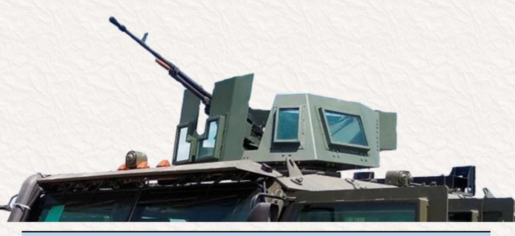
A weapon station is protection against being hit by enemy small arms and different explosive devices. It allows the crews of combat vehicles to conduct fire under armor protection in manual or automated mode.
