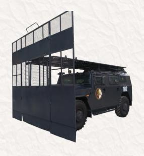
Barrier and assault equipment "Kalkon" provides shield for frontal protection of personnel and vehicles from the effects of various hard and heavy objects according to 0 class of protection.
