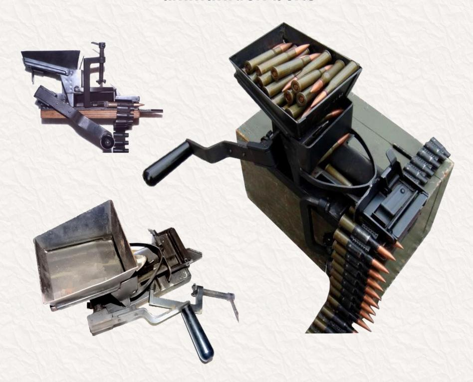
Rakov belting device is used for fast belting of a machine-gun belt. Cartridges are bulked into the bunker, turned over by rotating the handle, stacked and belted into an ammunition belt moving it forward.
